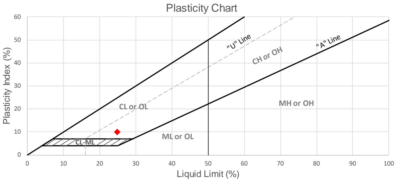
Atterberg Limits Test – ASTM D4318
